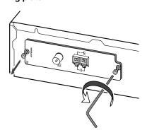
3 Screw the supplied removal thumbscrews into the two holes just below the holes that were used by the hexagonal socket head screws. Screw them in about 3/16" (5 mm). Hold and pull both of the thumbscrews to remove the board.
